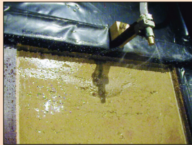
Figure 11 – An SRE test wall being exposed to pressure-driven water penetration testing in the climatic simulation chamber at Sheffield Hallam University (© Hall M)
